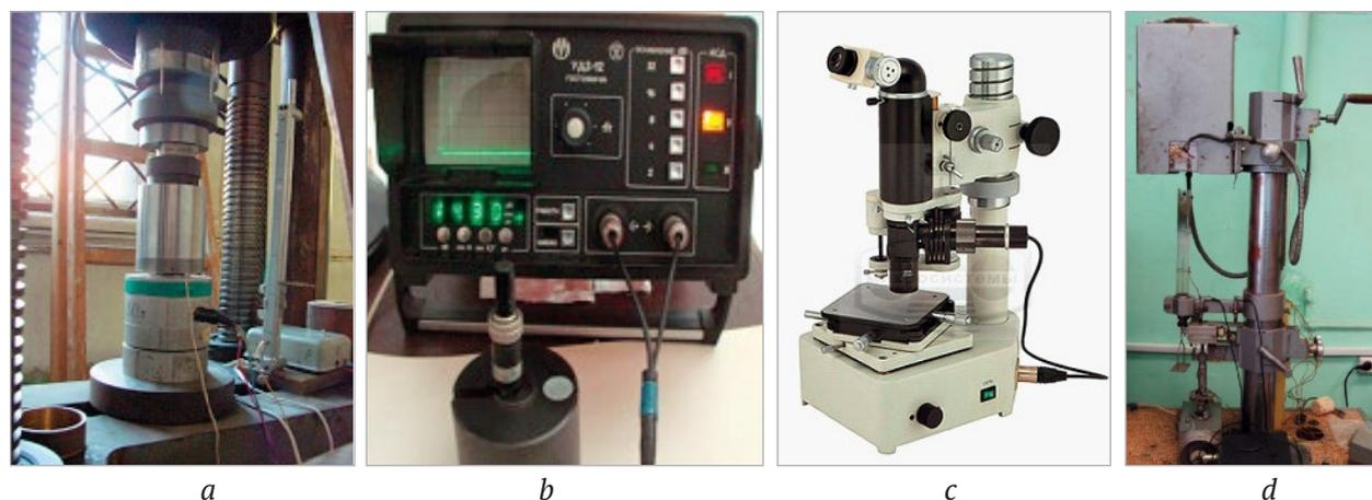
Figure 2. Equipment applied to measure the main borosilicate glass quality indicators: a – GMS-50 press, b – UD2-12 flaw detector, c – PMT-3 microhardness meter, d – Klyuev-Chernousov system quartz dilatometer-viscometer
