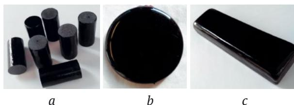
Figure 1. Glass samples for various testing methods: a – compressive strength and Young's modulus; b – bending strength and heat resistance; c – coefficient of linear thermal expansion
