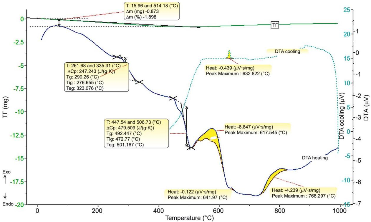
Figure 3. Thermogram for BSS-20 borosilicate glass sample
