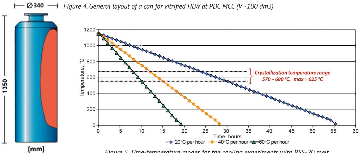
Figure 5. Time-temperature modes for the cooling experiments with BSS-20 melt
