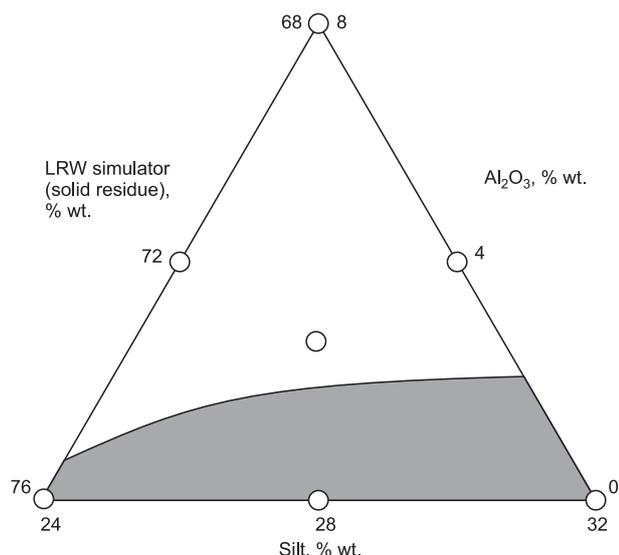
Figure 2. Areas of raw mix compositions for cement compound production
