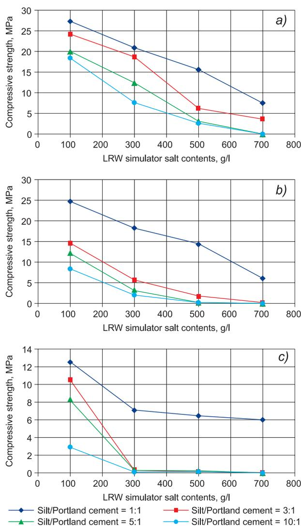
**Figure 1. Strength characteristics of cement compounds on the 28th day of hardening obtained for different Solution/Binder ratios: a) S/B = 0.4; b) S/B = 0.6; c) S/B = 0.8**
