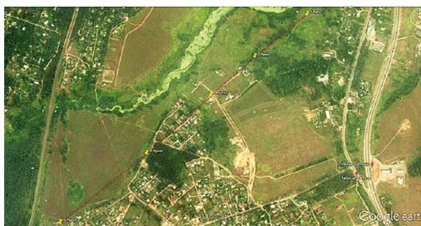
Fig. 3. Reference basis of the Federal Center for Geodesy, Cartography (Moscow Region). The red lines represent the basis lines. Yellow markers represent equipment installation stations
