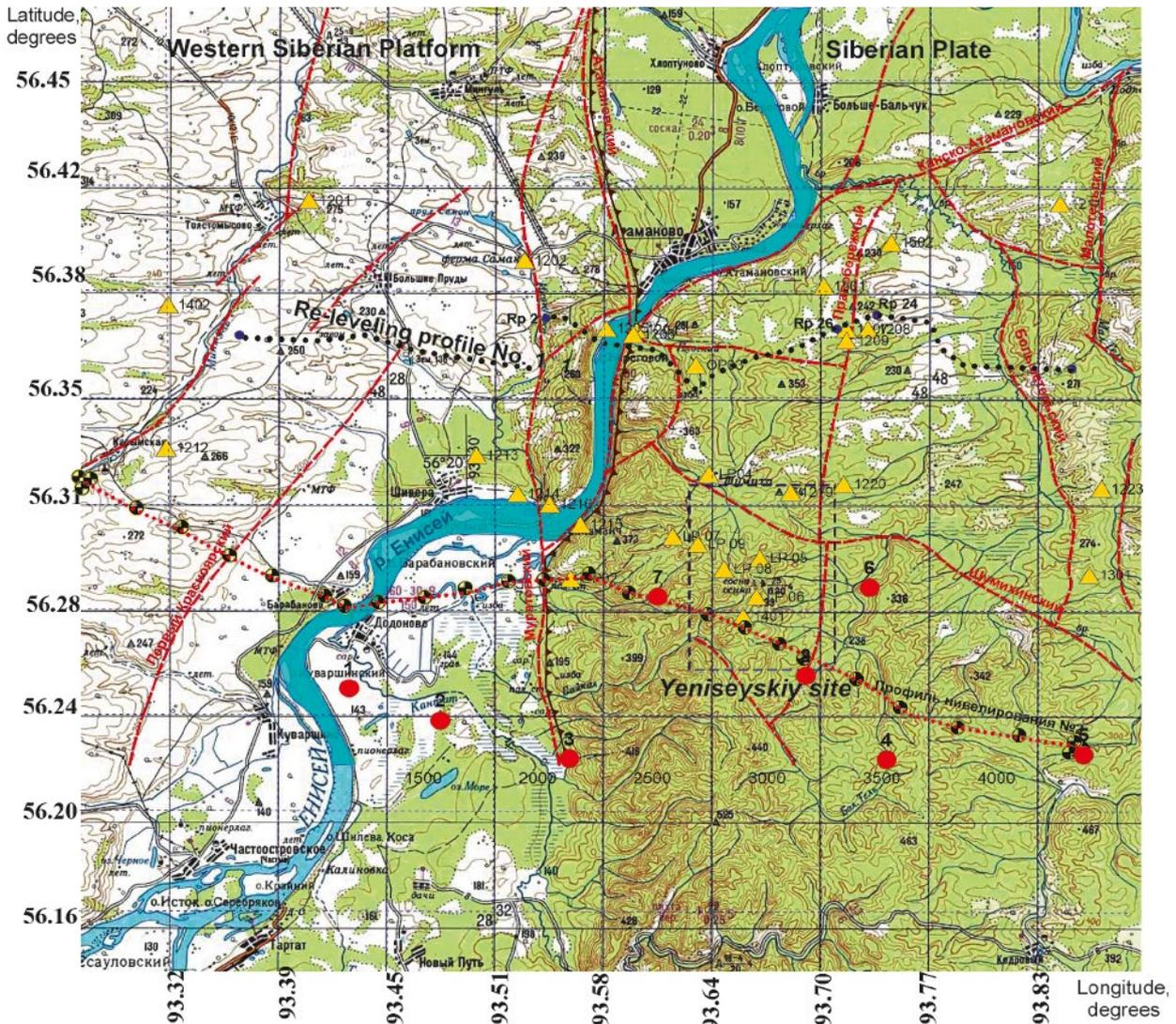
Fig. 2. Geodynamic observations in 2019-2024 The yellow triangles represent the existing GNSS stations, the red circles – new GNSS stations, the black dotted line – existing re-leveling profile No. 1, the red dotted line represents the new re-leveling profile No. 2
