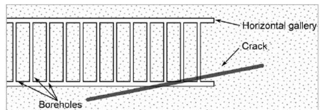
Fig. 2. Layout of dead-end boreholes
