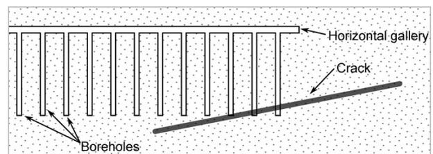
Fig. 3. Layout of open-end boreholes
