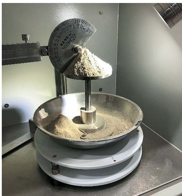
Figure 1. Natural cone angle measurements for sample No. 6 using a universal powder analyzer PowderPro M1
